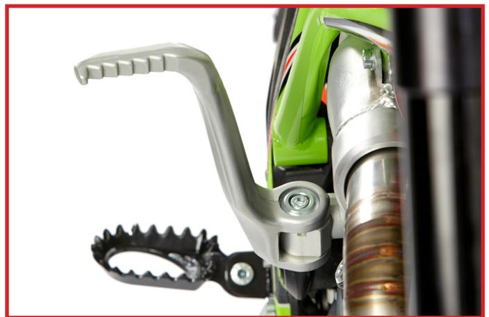
On this 2018 model Vertigo has also implemented several changes in the geometry system of the kickstart pedal. That will provide further ease during the starting process. Alongside with it, the Vertical features a reinforced sidestand, which will bring better stability and security when the bike is stopped.
